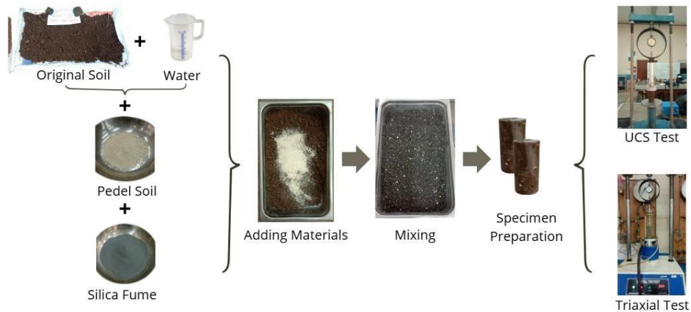
Figure 4. Specimen preparation and laboratory testing
