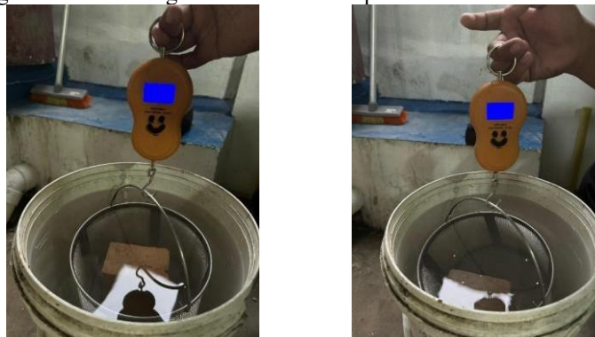
Picture 9. Pseudo-density testing process
