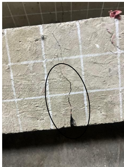
Figure 3. 8 Patchwork Concrete Fracture with Bridging Effect
