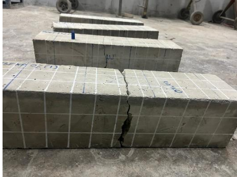
Figure 3. 7 Concrete Breaks Without Patchwork
