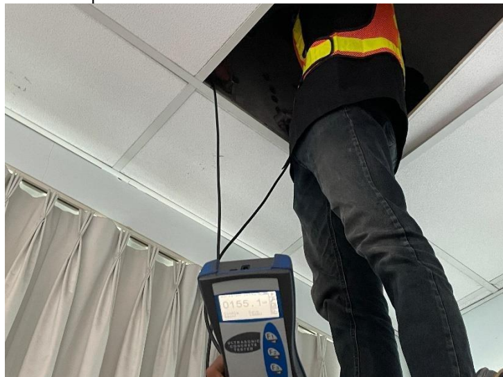
Fig. 5. Sample Testing of Ultrasonic Pulse Velocity Tool
