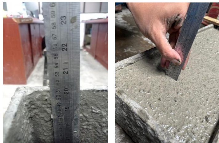
Fig. 4. Implementation of the H1 L-Box Test
