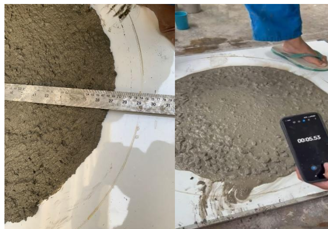
Fig 2. Slump-Flow Test Procedure
