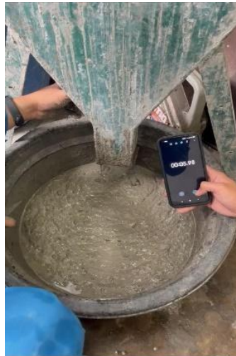
Fig 3. Implementation of the V-Funnel Test
